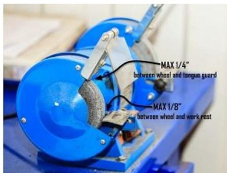
Adjustments to the work rest or the tongue guard must never be made while the wheel is in motion. Ensure the work rest and the tongue guard are tightly secured after each adjustment. Because the wheel wears down over time, it is important that both the work rest and the tongue guard are regularly checked and adjusted.
